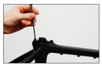
5.) Re-install the seat post and the seat post clamp. Tighten the seat post clamp bolt on the ISO FLEX insert. Clamping the seat post in a bike stand can make the process easier.
