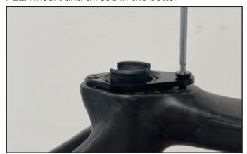
5.) Torque the Top Cap Bolts to 5 Nm.
