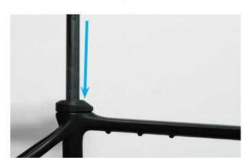
10.) There is an opening in the Rubber Cap to access the Seat Post Clamp screw. Torque the Seat Post Clamp Screw to 5Nm.
