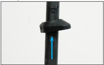
8.) Apply some grease to the seat tube and insert the seat post into the frame.
