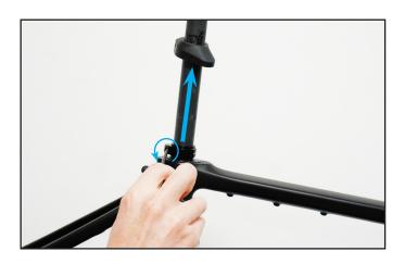
3.) Slide the Seat Post Clamp up off the ISO FLEX insert to access the Top Cap Bolts.
