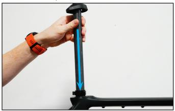
9.) Slide the Seat Post Clamp Rubber Cap down over the Seat Post Clamp.
