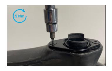
6.) Install the Seat Post Clamp on the ISO FLEX insert.
