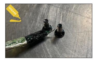
4.) Place the Seat Post Top Plate over the ISO FLEX insert and thread in the bolts.
