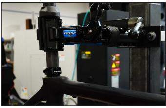
6.) Pull down on the frame to remove the ISO FLEX insert from the frame. This is a tight fit and may require some rocking the frame back and forth to release it from the frame.
