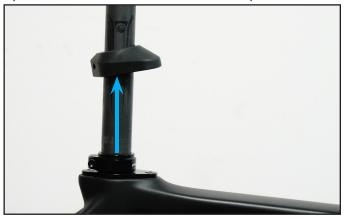
2.) Loosen the Seat Post Clamp Screw with a 4mm hex wrench and remove the seat post.
