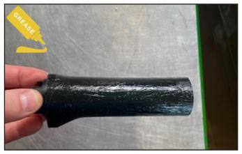
2.) Gently press down on the ISO FLEX insert to place it down into the frame.
