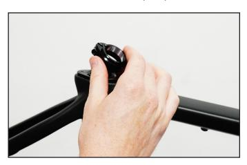
4.) Loosen and remove the Top Cap Bolts and the Top Plate.
